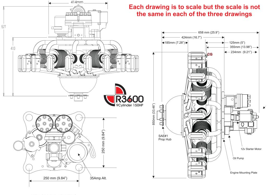
VIEW OF REAR MOUNTING PLATE AND BOLT ON ACC'S
