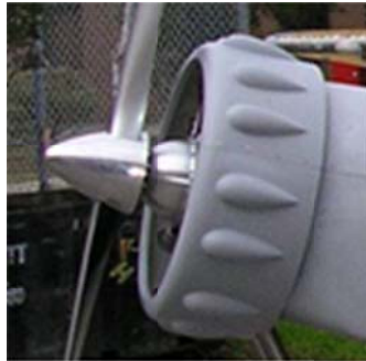
Gap between fuse & Cowl
