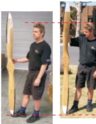
Left R2800 prop 76" x 55" Rotec wood laminated prop
