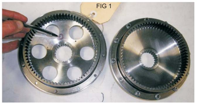
Rotec recommend inspection of the bell gear and PSRU on all engines, irrespective of the type of carrier plate, as such inspections provide a visual representation on the health of the engine, oil distribution and wear patterns.
