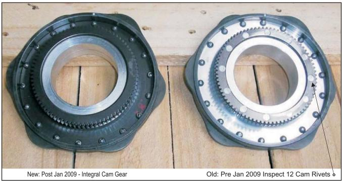
The cam on the right is the standard cam assembly and is typical of all engines up to January 2009.
