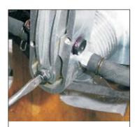
Valve adjuster screw used to set valve clearance.
