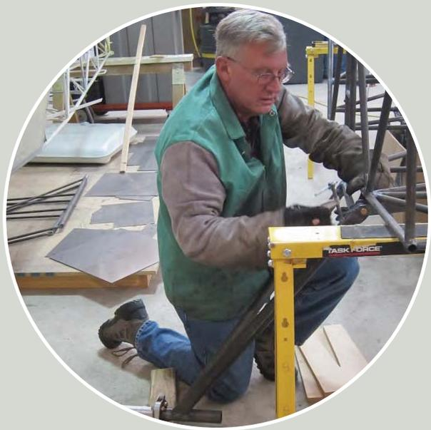
buy most of the required tubing and start on the fuselage. Today, February 2011, most of the basic frame is welded as is the elevator, horizontal stabilizer and fin. Landing gear and Rudder fabrication are next.
